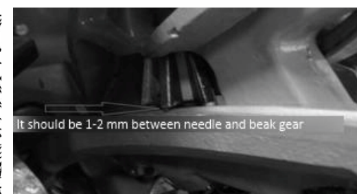
Figure 34: Needle setting
